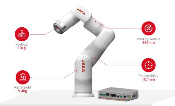
The JAKA Minicobo is compatible with Ethernet protocols (TCP/IP) and control interfaces such as Modbus and Profinet. It can simply and quickly integrate end effectors, grippers, suction, vision systems and force control modules. JAKA also provides an ROS package and SDK secondary development package, meaning that operators can quickly adapt the cobot to suit new or experimental applications.
